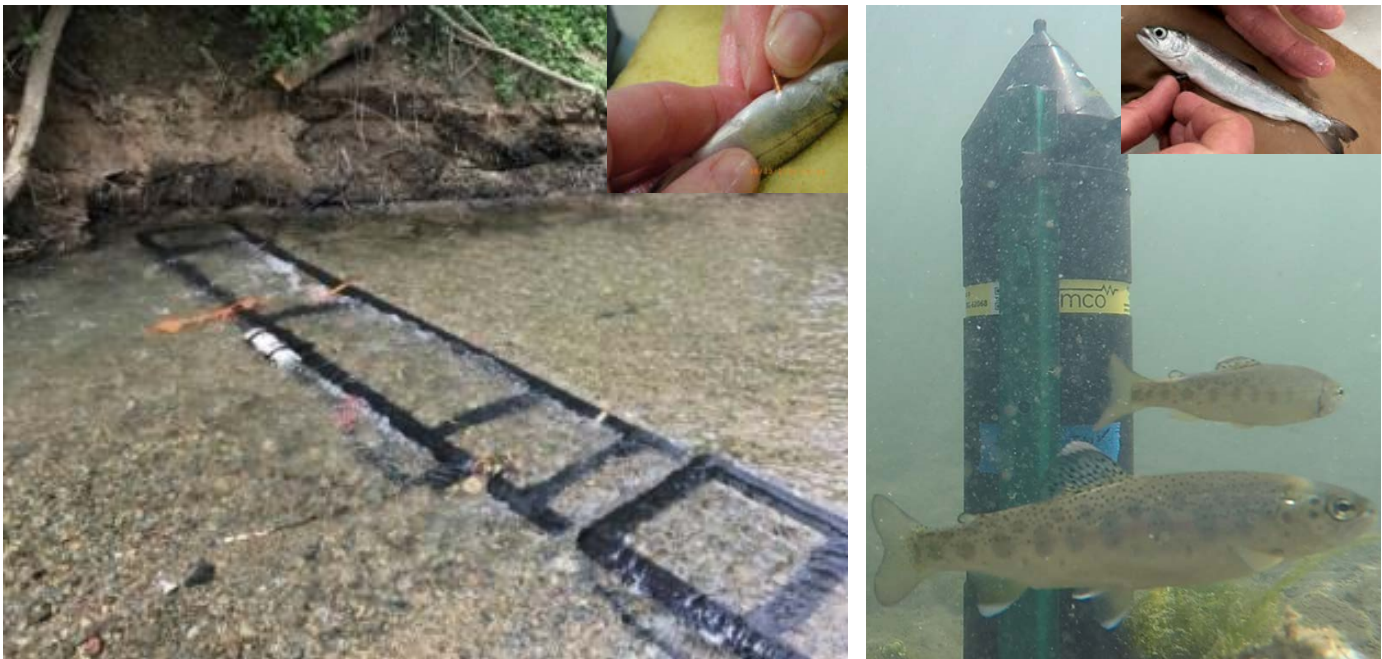
PIT tagging procedure and PIT antenna (left photo) and acoustic tagging procedure and acoustic receiver (right photo).
